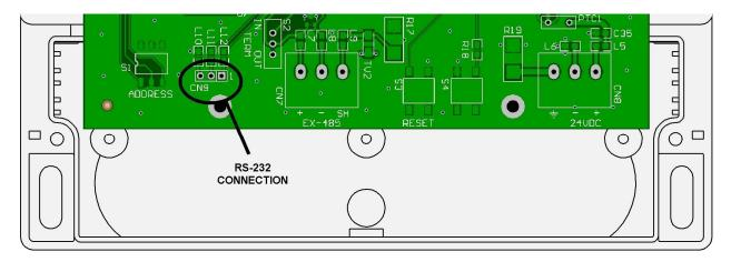
This 3-pin connection (CN9) is only a temporary connection and should not be permanently wired. See the Firmware Updates section for more information about the use of this connection.
