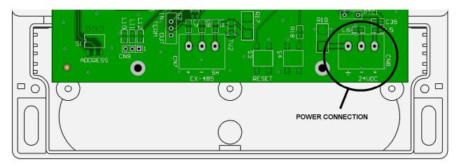
The power connection (CN8) is a three wire terminal block located on the far right. Two terminal screws marked + and – are for connecting to an isolated 24VDC power source. A 14 or 16 AWG wire would be sufficient for these two power connections.
