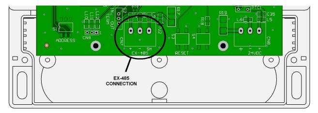
The EX-485 connection (CN7) is a three wire terminal block located near the center of the printed circuit board and is for connection to the RS-485 expansion network. Two terminal screws marked + and – should be connected to the positive and negative wires of the expansion network cable. The third terminal screw marked SH should be connected to the shield of the expansion network cable. Do NOT connect the shield to earth.
