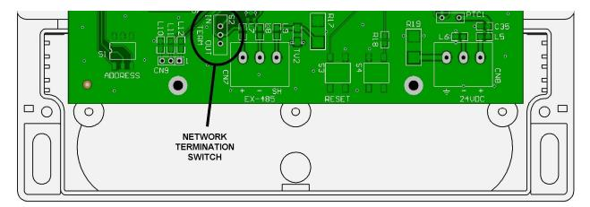
If the expansion console is located at the end of the network cable the network termination switch must be switched IN, otherwise it should be switched OUT. The termination switch is labeled TERM and located under the lower compartment cover near the EX-485 terminal. Additional information is available under Section 3.4.2 EX-485 for Expansion Network and under Section 3.5 RS-485 Network Requirements.
